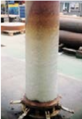
Ni-base ingot produced in VAR operation
