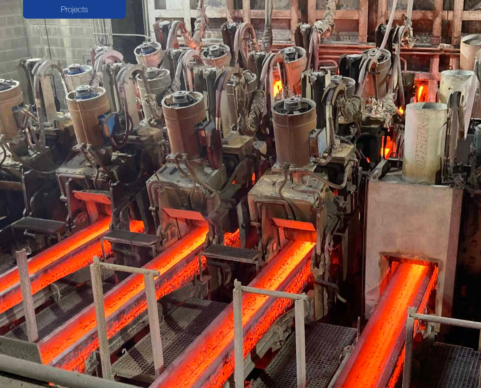
Revamped beam blank caster already in operation at this European confidential customer
