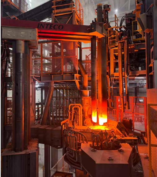
60t electric arc furnace (right) and ingot casting facility (left) in operation at GMTC
