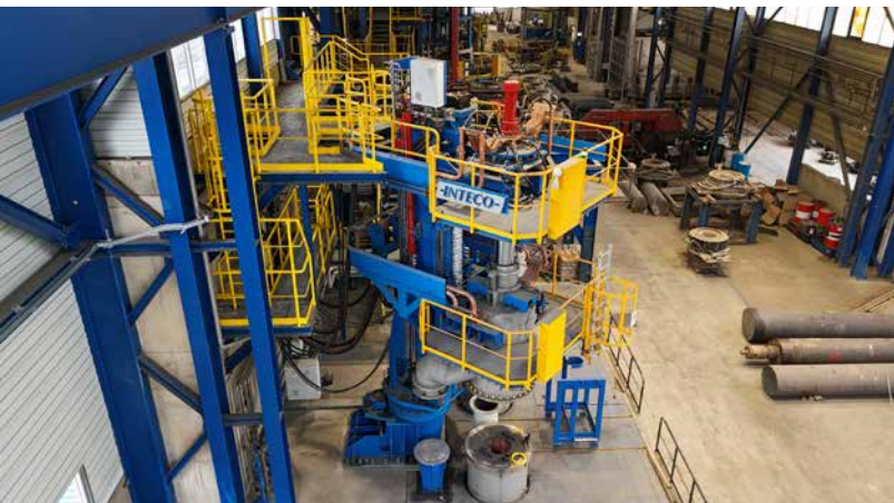
Breitenfeld Edelstahl industrial area & 16t VAR furnace (left), 12t VAR furnace at SeAH Specialty Steel (right picture)
