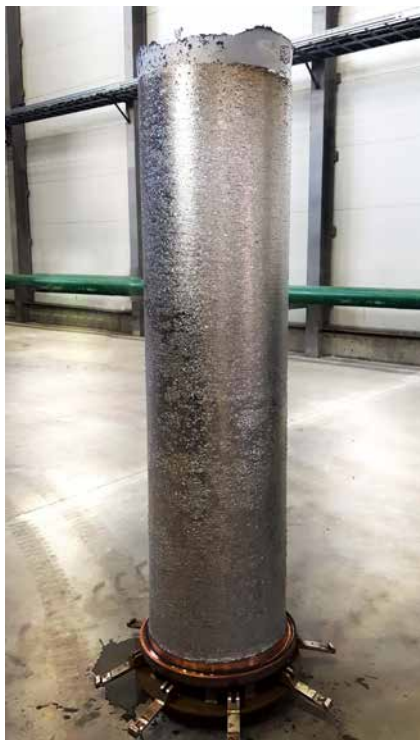
Titanium ingot produced by an INTECO TI-VAR
