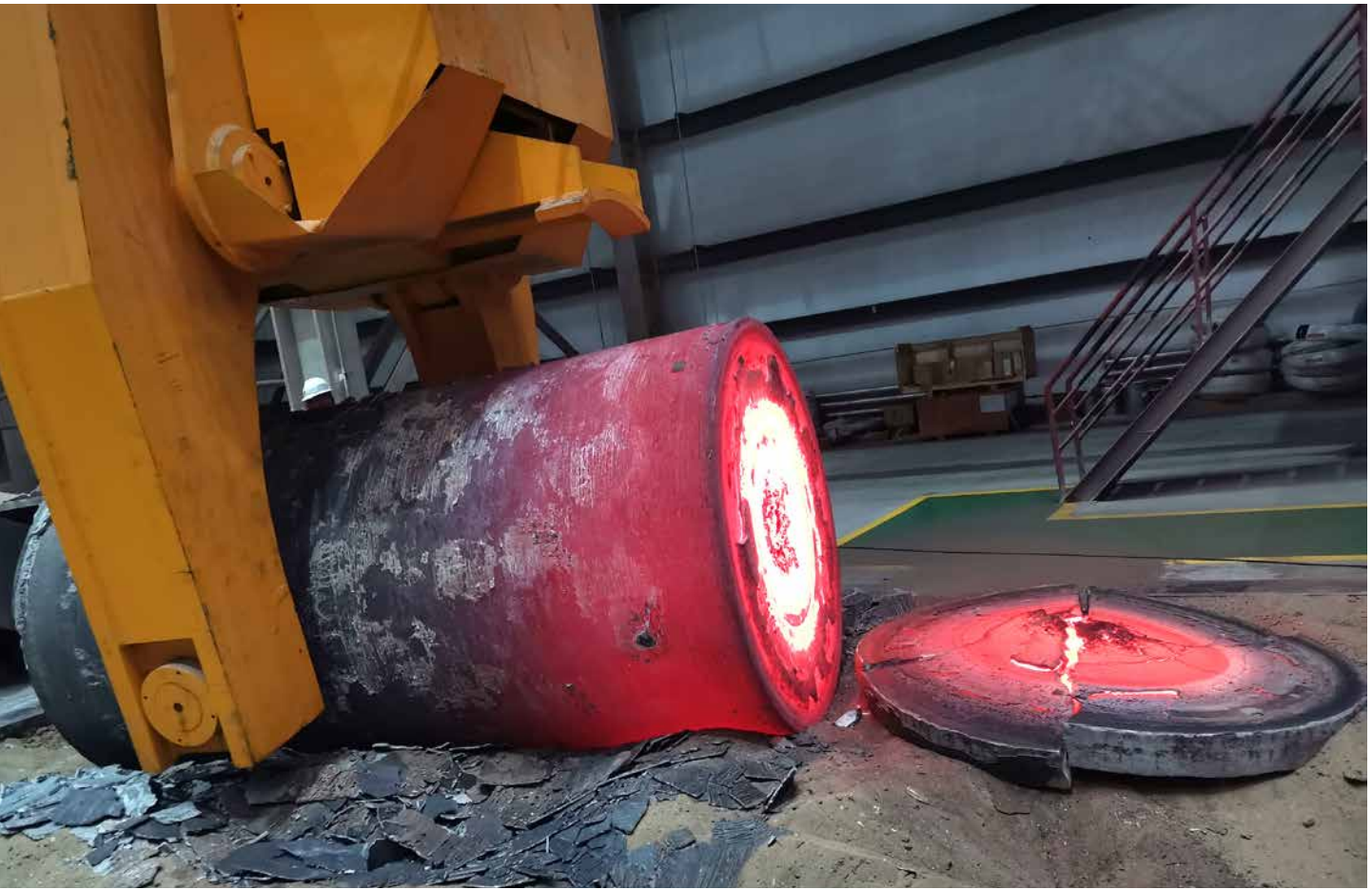
Super-sized ingot produced by the 160t ESR furnace
