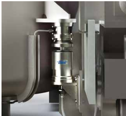
Automatic stirring gas supplied by INTECOS automatic gas coupler systems guarantee operator safety.
