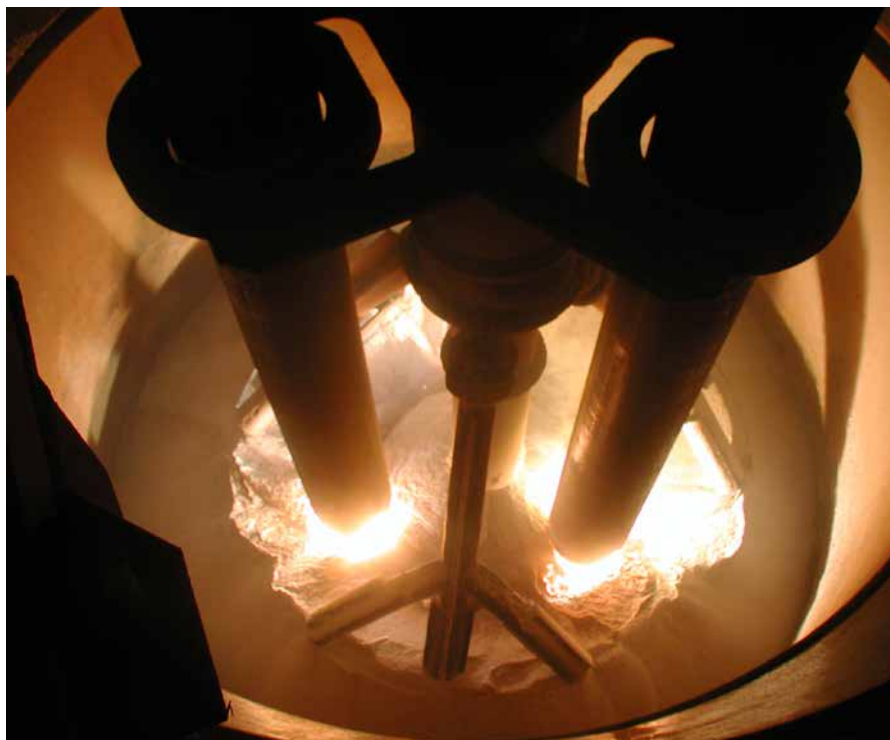
View insight a fused magnesite furnace from a previous project
